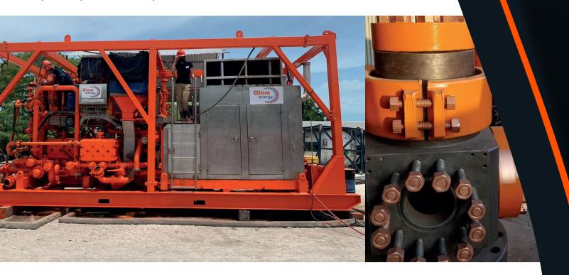
Hammer Unions are manufactured according to the requirements of the service in different diameters, with capacities up to 20,000 PSI of working pressure. Unions for nitrogen gas or acid fluid service are manufactured in accordance with NACE MR-01-75 and API RP-14E. Our lines and accessories have traceability and maintenance to guarantee safety in operations.
